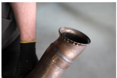
Carefully remove the metal gasket from the end of the OE exhaust where it joins to the downpipe and reinstall on the Scorpion Front Pipe
